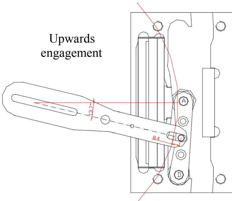
As a suggestion for the safety gear fixing to the sling, the tightening torque of 8.8 M12 screws is 79.09 Nm and 111 Nm for those of 10.9.
